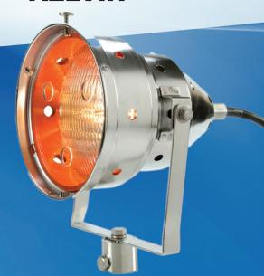
The BIRNS Kelvin<sup>™</sup> is a powerful 16,000 lumen tungsten halogen floodlight that is trusted worldwide in major nuclear power stations. This proven system requires no costly radiation-sensitive electronics. It is seismically qualified per IEEE-344, and with its rugged stainless steel housing and a Lexan polycarbonate protector, it enhances safety and performance in a range of demanding nuclear illumination applications.
