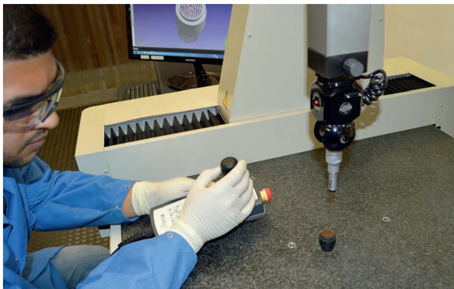
Above: A technician inspects a Millennium 3P connector insert with 83 electrical pins with BIRNS' CMM. Below: A custom titanium fixture for testing Millennium 3P FR titanium connectors to withstand pressure for oil filled cable assemblies
