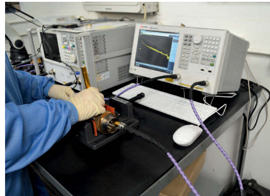
High-frequency RF testing is conducted with an ENA series network analyser
