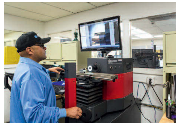
A BIRNS quality team member inspects a connector insert with a digital video comparator, which combines the capabilities of a horizontal optical comparator and a vision metrology system
