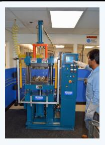
We recently enhanced our existing molding capabilities with the addition of a new custom 40 ton hydraulic transfer press. It will provide additional firepower to BIRNS' molding facility for connector inserts, allowing computer controlled precision for functions like injecting glass reinforced epoxy (GRE) and providing increased speed and output for large orders.
