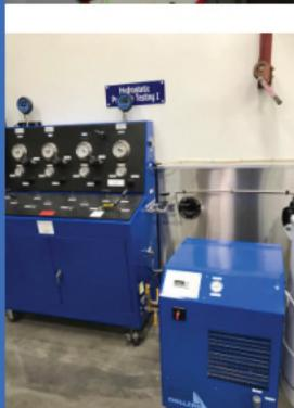
The new cold hydrostatic pressure testing provides automated, programmable multiple pressure cycles with real time data recording of electrical and optical testing, along with digital output of pressure and temperature data. It was initially developed to meet customer requirements for a new BIRNS Millennium™ 6km-rated hybrid electro-optical pin configuration, the 3O-1F3.
