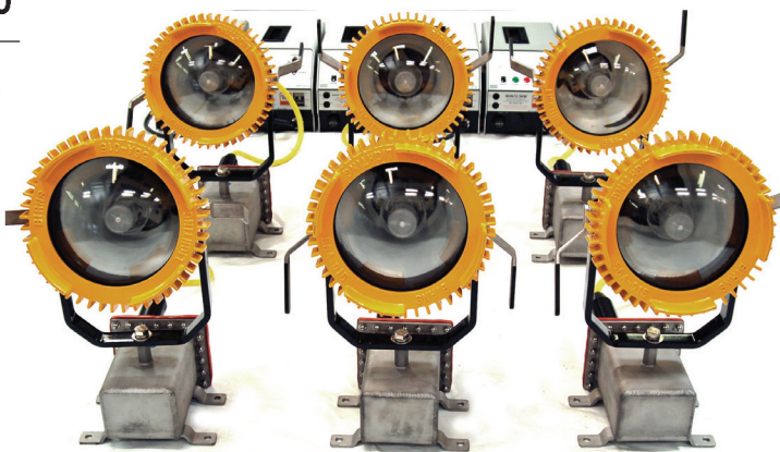
BIRNS developed custom HMI lighting systems for the Costa Concordia salvage project. These 380,000 lumen, 4-kW systems were used during the complex and several month long project to provide underwater illumination of up to 50 ft away at night.
