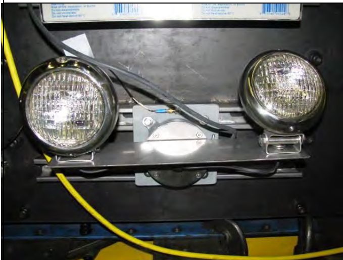
4634 unit with incandescent lamps and Triax Accelerometer mounted
