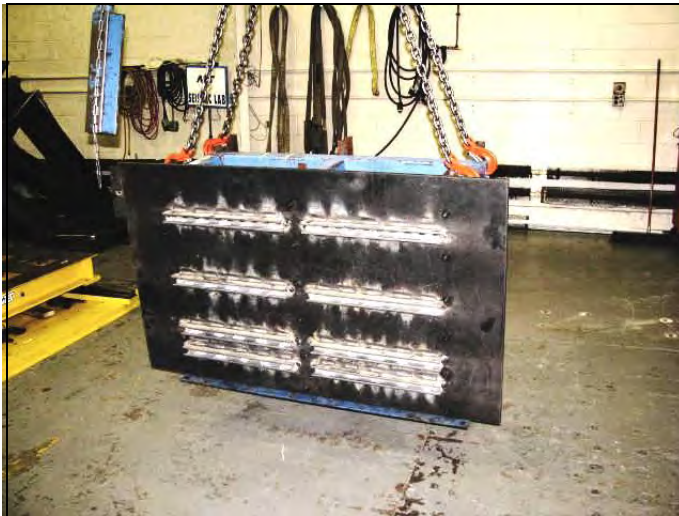
Unistrut channels welded to vertical plate Front view of fixture
