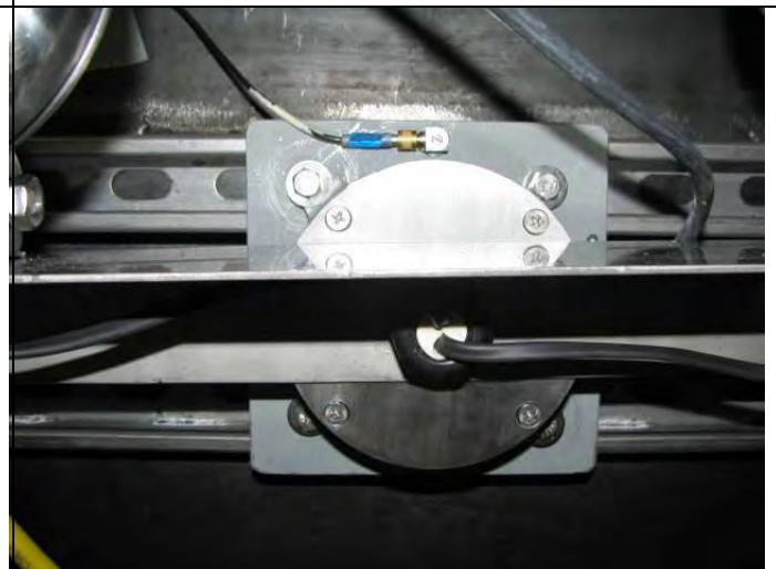
Triax accelerometer mounted on plate of 4634 unit
