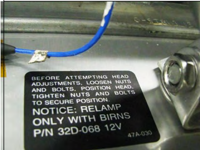
Topside markings on 4702 ELU S/N 100015
