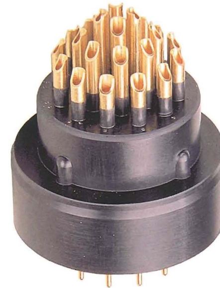
BIRNS solder pots with 15-degree lead-in O-ring chamfer built into insert. Each solder pot is insulated part of its length with a layer of moulded GRE. After wire termination, heat-shrink tubing covers the insulated GRE area, ensuring a completely insulated termination and eliminating possible electrical interference between pins
