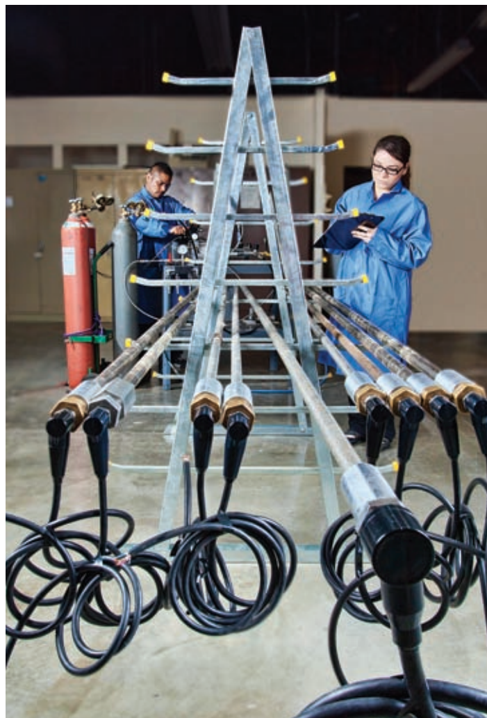
Final helium pressure testing with MIL-L-25567 compliant gas leak detector
