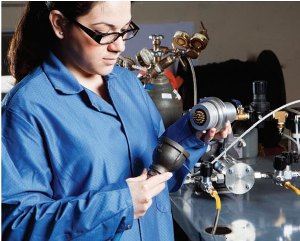
BIRNS P38100-24-RA-LS penetrator insert is mated to custom fixture for helium pressure testing
