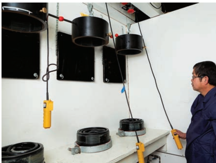
Left: Continuity and insulation resistance testing of entire penetrator. Right: Multiple penetrators in tanks for six-cycle saltwater hydrostatic pressure testing at 1250psi, with concurrent IR testing
