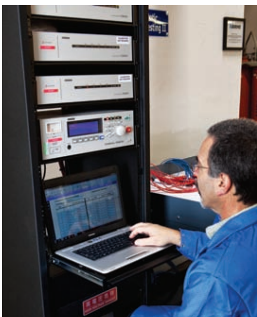
Left: Continuity and insulation resistance testing of entire penetrator. Right: Multiple penetrators in tanks for six-cycle saltwater hydrostatic pressure testing at 1250psi, with concurrent IR testing
