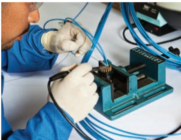
Twenty-four cable conductors are soldered to inboard and outboard sides of the penetrator's insert
