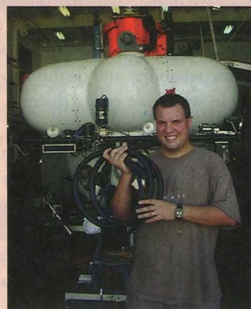
Happy 2000 HURL Chief ET Chris Taylor with the new BIRNS 40-conductor, metal shell, man-rated cable assembly.
