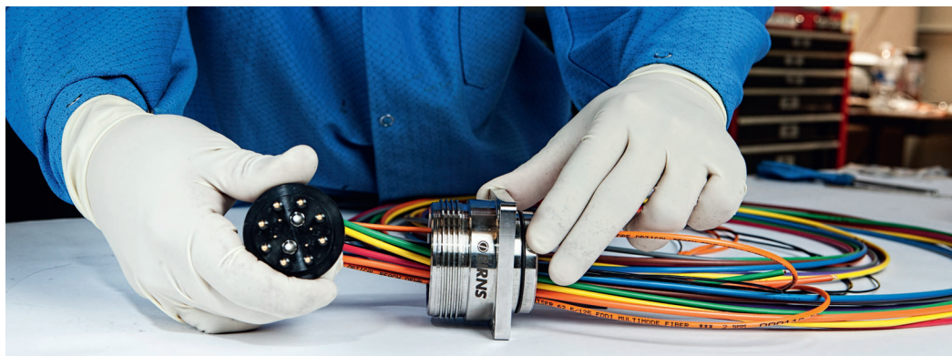
Development of a custom electro-optical cable assembly with two multimode optical fibres, eight 2.5kV conductors and four 600V conductors for the US Naval Facilities Engineering Command/Engineering Service Center
