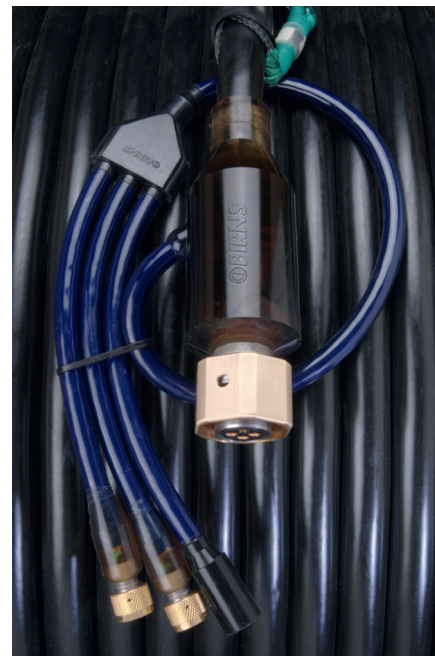
Rugged BIRNS cable assembly for the IceCube Neutrino Observatory in the South Pole: a high-power BIRNS Primus connector with four 2 AWG contacts for the hot-water drill pump at depths of 1.5km to 2.5km in the ice cap, and BIRNS Millennium 3G connectors for its temperature and pressure sensors
