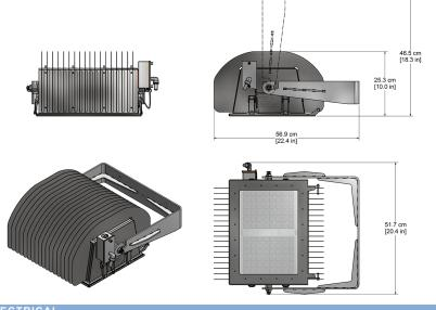
ELECTRICAL Mains Input (VAC): 110-277 Frequency: 50 Hz or 60 Hz Power: 210W Power Factor: .96
