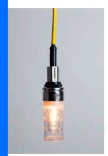
The BIRNS TubeLight™ delivers powerful 10,000+ lumen brilliance for 360° underwater drop-light use in confined spaces. It's compact (only Ø48mm) and versatile (100W to 500W) with a wide range of accessories to tailor it to a variety of demanding nuclear applications. It operates at up to 300M, and has a sturdy stainless-steel construction.
