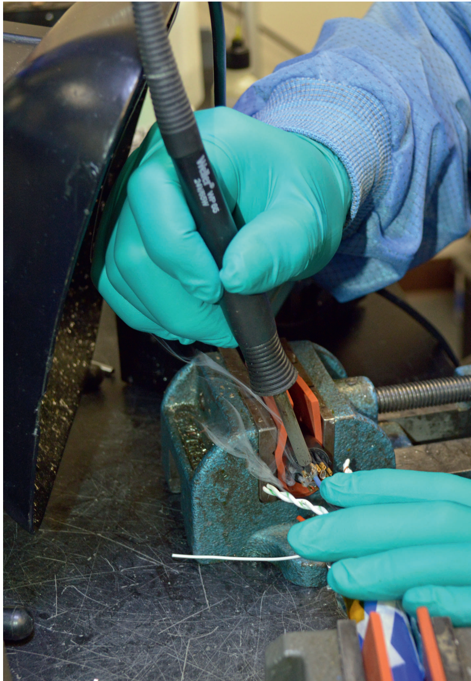
Special termination protocols were developed for BIRNS' exclusive 52A-278 cable constructed for Cat 8.2 use
