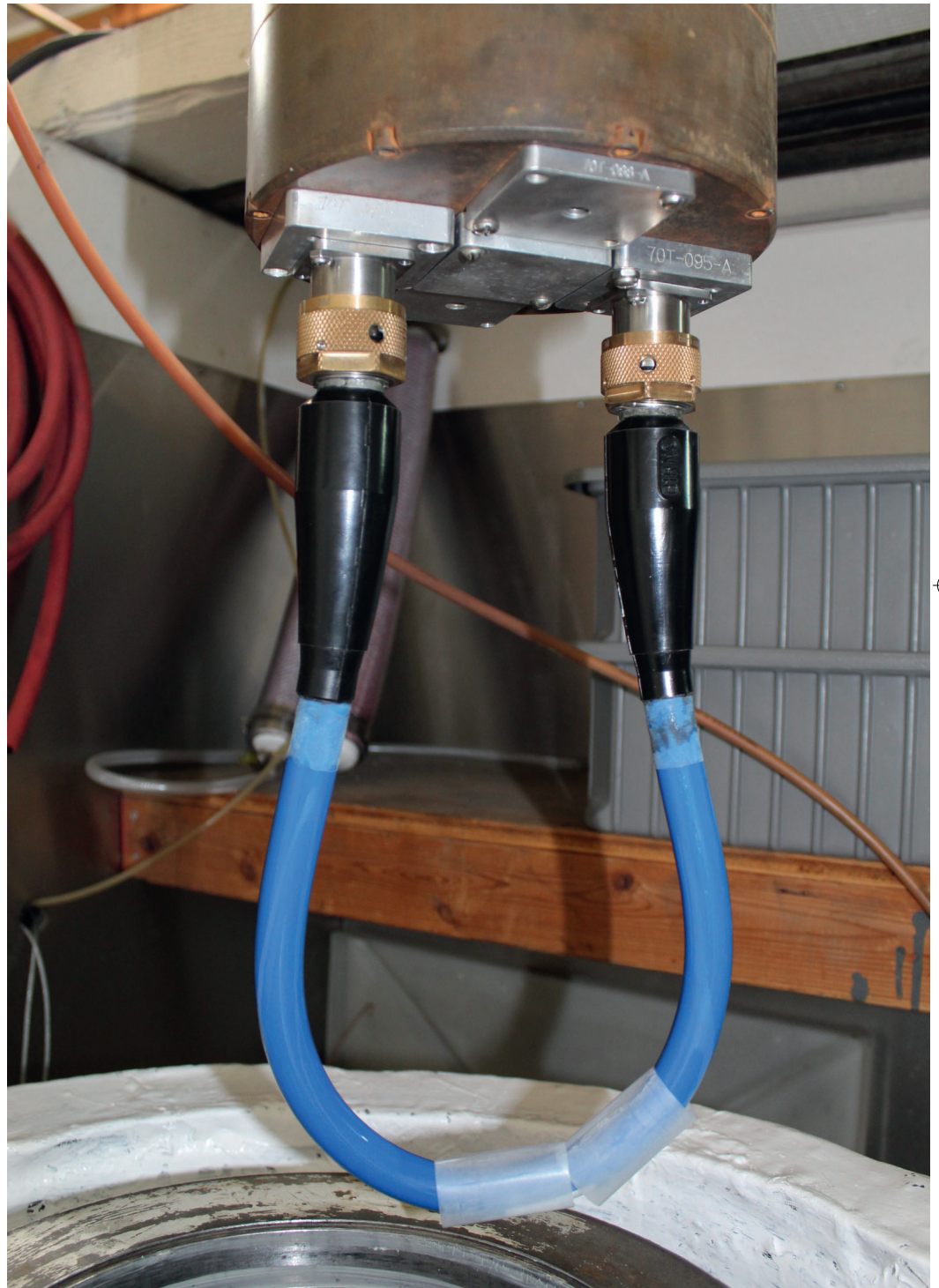
The cable assembly is attached to flanged receptacles mounted inside a high pressure hydrostatic test chamber
