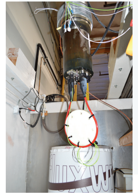
» A BIRNS 30-1F3 cable assembly during unique extreme cold, extreme depth testing at 6 km in a controlled 2°C (±1°C) environment. (Photo credit: BIRNS)
