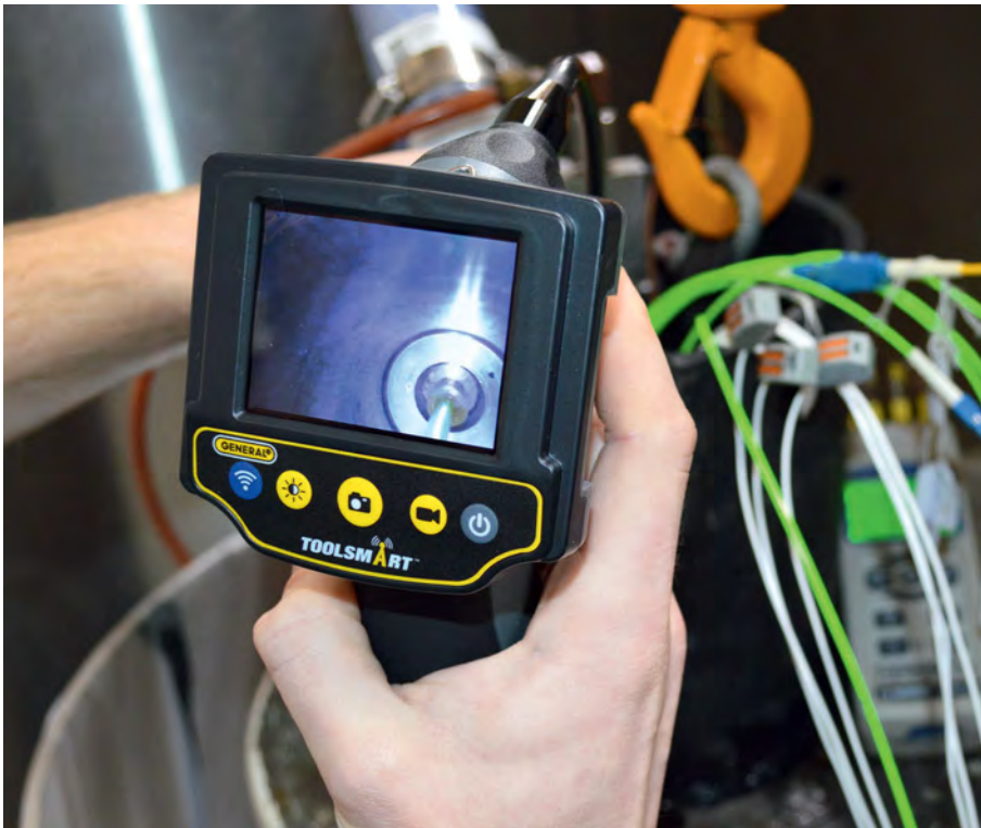
A Wi-Fi connected video inspection camera provides visual monitoring for moisture intrusion and condensation on the inboard side of the connectors, while under test pressure and temperature
