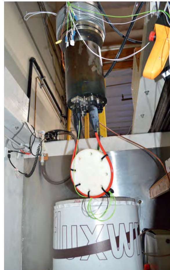
BIRNS developed a new extreme cold, extreme depth pressure testing system that allows 48-hour-plus continuous testing of connectors and cable assemblies at six kilometres in a controlled 2°C ( \pm 1^\circ\text{C} ) environment
