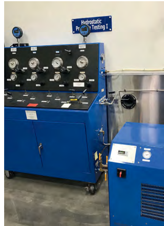
The new pressure testing provided automated, programmable multiple pressure cycles with real-time data recording of electrical and optical testing, along with digital output of pressure and temperature data
