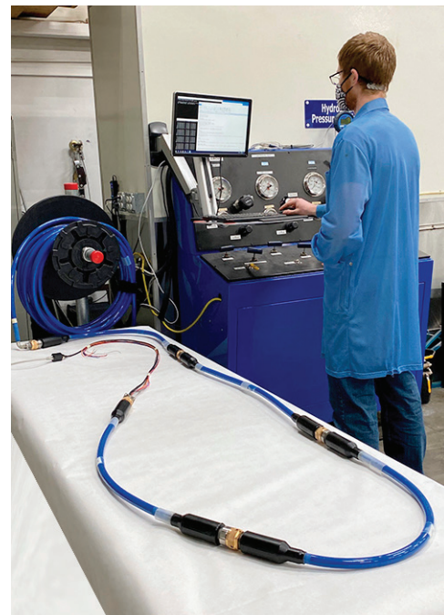
9.48 Gb/s over 20m (65 ft.) of cable with five inline mating pairs.
