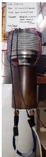
Setup for the Gigabit data transfer test under pressure requirements
