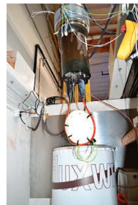
Low temperature/high pressure test capability simulates actual conditions at depth, with long-term continuous pressure testing in a controlled 2°C ( \pm 1^\circ\text{C} ) environment; programmable, automated multiple pressure cycles; real-time electrical and optical test data recording; and continuous digital output of pressure and temperature data.
