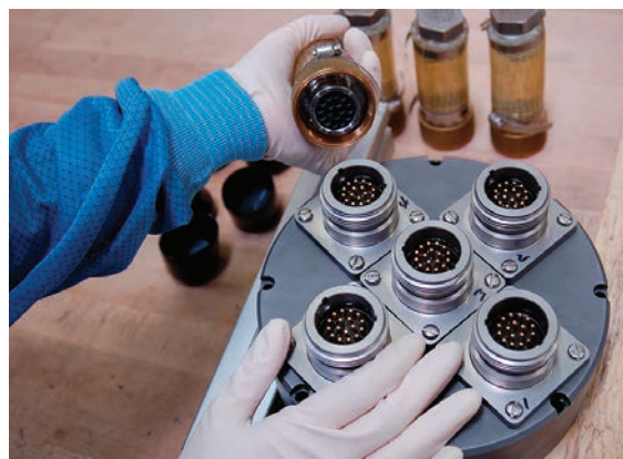
Preparing various inserts for high-pressure open-face hydrostatic testing.
