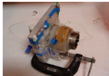
After the test is completed, the BIRNS connector is embedded in ice...but still transmits optical signal.
