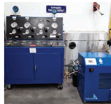
The pressure system controls located outside Hydrostatic Pressure Testing facility I (The chiller was not used for this test.)
