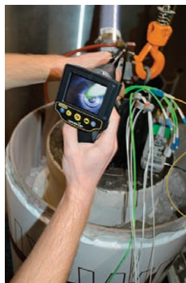
Low temperature/high pressure test capability simulates actual conditions at depth, with long-term continuous pressure testing in a controlled 2°C ( \pm 1^\circ\text{C} ) environment; programmable, automated multiple pressure cycles; real-time electrical and optical test data recording; and continuous digital output of pressure and temperature data.
