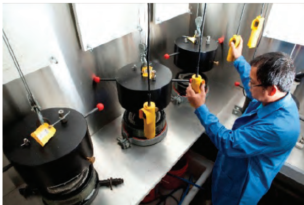
BIRNS' custom-engineered programmable hydrostatic system has automated digital data recording capabilities. It can simultaneously run three independent pressure circuits in six chambers at pressures up to 20,000 PSI (138 MPa), in fresh or salt water.
