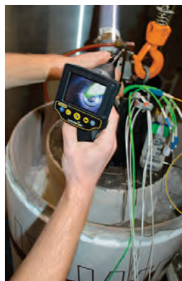
Low temperature/high pressure test capability simulates actual conditions at depth, with long-term continuous pressure testing in a controlled 2°C (±1°C) environment; programmable, automated multiple pressure cycles; real-time electrical and optical test data recording; and continuous digital output of pressure and temperature data.
