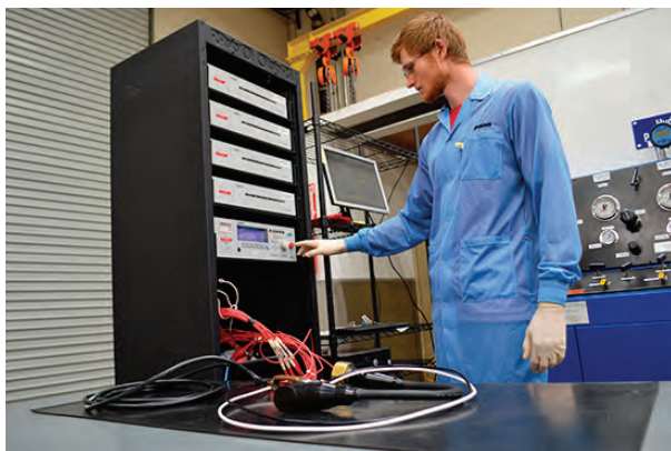
Final acceptance tests using a Kikusui TOS9213S DC DWV/IR Tester with high voltage scanners. Our custom-made programmable system permits simultaneous testing of up to 16 electrical circuits at voltages up to 6kV, even while under hydrostatic pressure.
