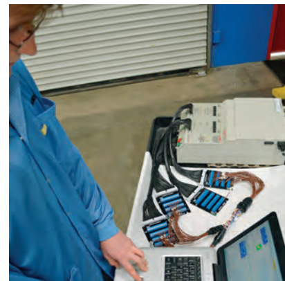
Testing of complex wire harnesses at voltages up to 2100VDC/1200VAC, with a CAMI 829A HVX-21 128-line test system meeting all IPC/WH-MA-A-620B electrical test requirements.
