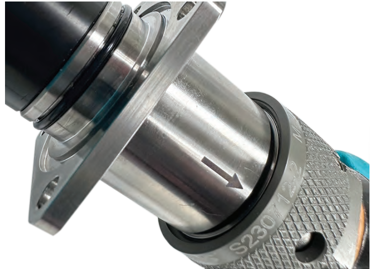
A mated M40 connector pair. The obscured fully-mated indicator band shows that the pair is properly mated.
